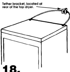
Attach both ends of tether located at the rear of the top dryer to a secured 2 x 4.
